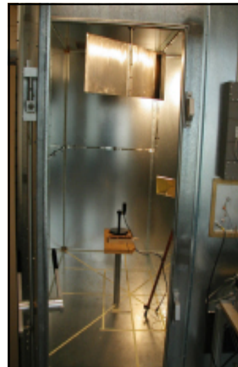
Reverberating chamber allowing the electromagnetic immunity of components to be tested as part of electromagnetic compatibility tests. Source CNRS
